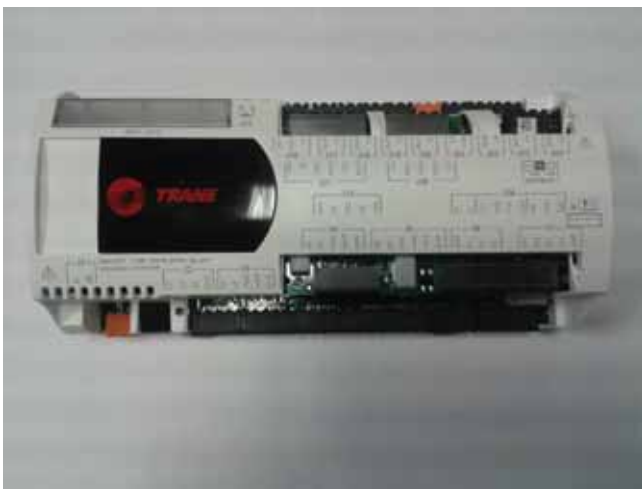
Figure 31 - CH536 main module
